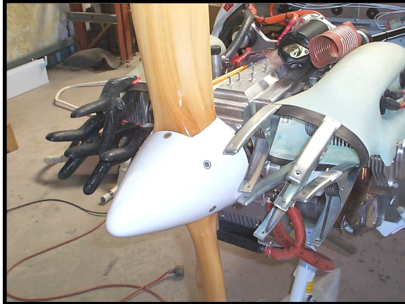
Clamp rubber while rubber is being glued.
